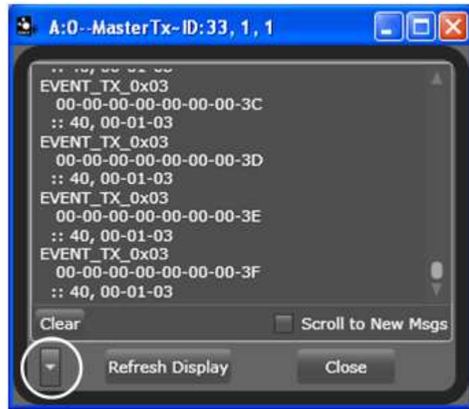
Figure 3 – 2. Pop-Out Window of Channel Feedback Display. Note there is an expander button (circled) in the lower left corner.
