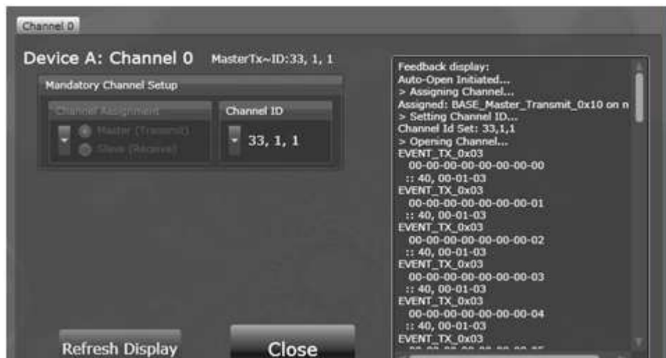
Figure 3 – 1. Channel 0 Configuration of Master Device
